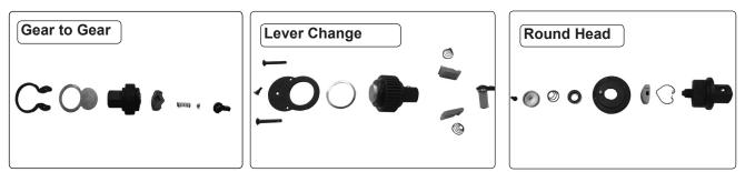
The head can be opened up to access the ratchet mechanism either by releasing the circlip using a pair of internal circlip pliers (fig.1) or removing the securing screws (figs. 2,3 & 4).
